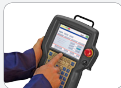
Integrated in the robot's teach pendant, the KempArc Browser allows you to set welding values without leaving the mechanisation application.
